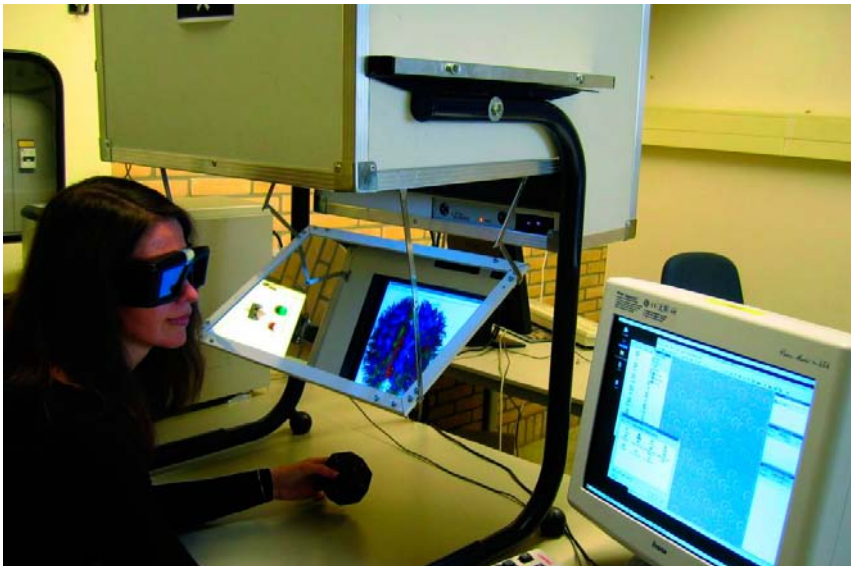
Figure 1: The Personal Space Station (PSS) offers stereoscopic visualization and direct interaction by means of tracked objects. Picture: UvA.
